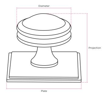
Fixings 1 x m4 x 30mm bolt Also available without a back plate or on a plain square back plate.
